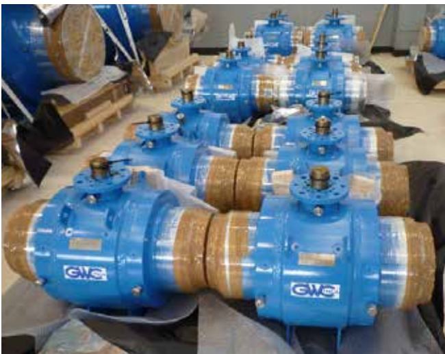
API 6D Trunnion Mounted Ball Valve Side Entry Welded Body 10" Class 600
