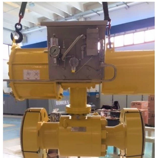
Pneumatic FC SDV 6" Class 2500 Side Entry Bolted Body
